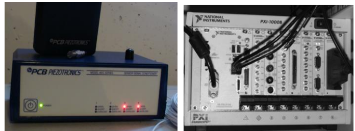
Figure 1: Left: High-speed pressure transducer (on top) and signal conditioning unit. Right: and fast waveform digitizer in PXI system.
